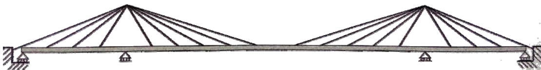
Figure 4 System C earth anchored cable-stayed bridge having a continuous deck throughout its length
