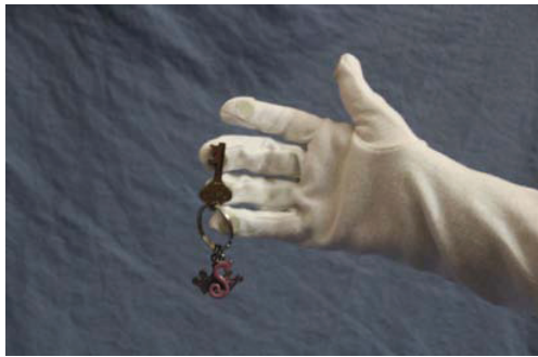
Fig3: The right glove- magnets help hold magnetic objects such as keys.
