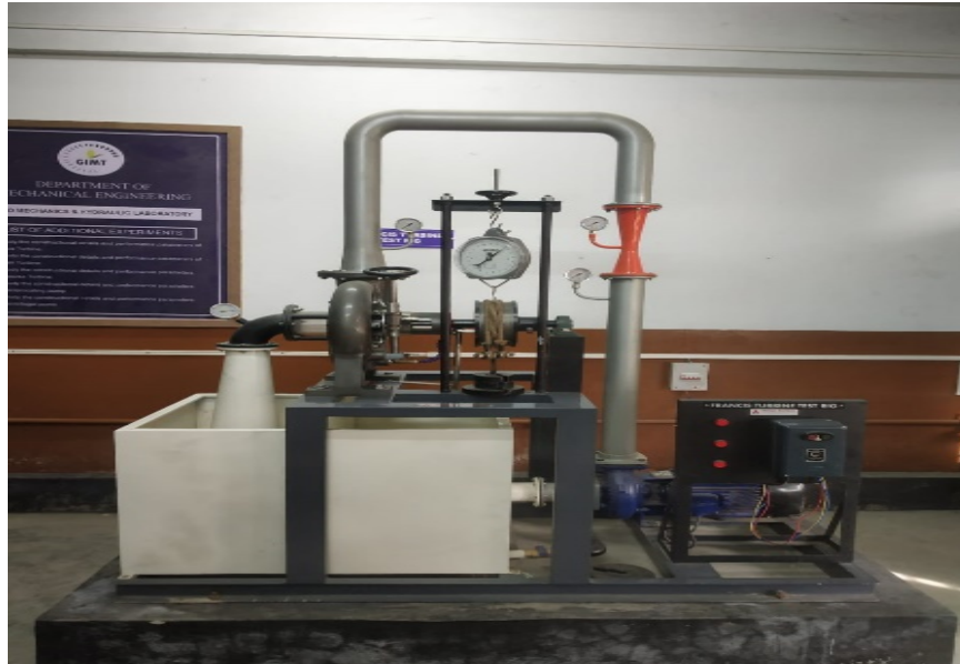
Fig.1 Francis turbine test rig
