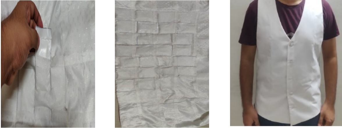
Fig 4: Cooling jacket incorporated with phase change material
