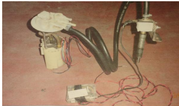
Figure 3: DeNOxation injection system
