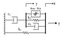
Figure 2- The modified Bouc-Wen model.
