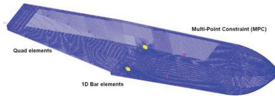
Figure 5. Meshing of Fuselage
