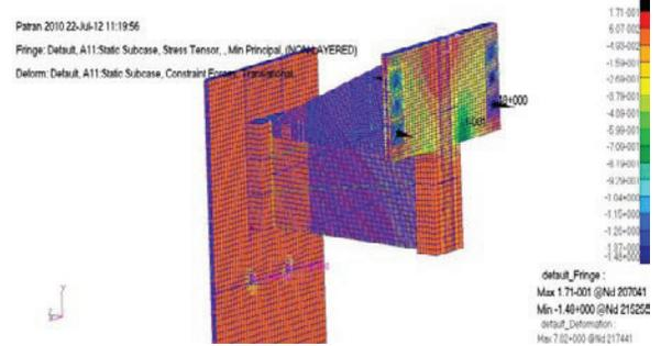
Figure 16. Min. Principal Stress of Vertical Fin
