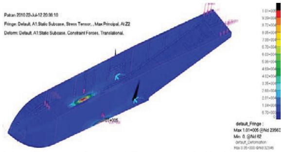
Max. Principal Stress of Fuselage is 2.68+004 MPa
