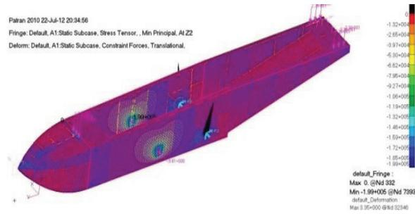
Figure 22. Min. Principal Stress of Fuselage
