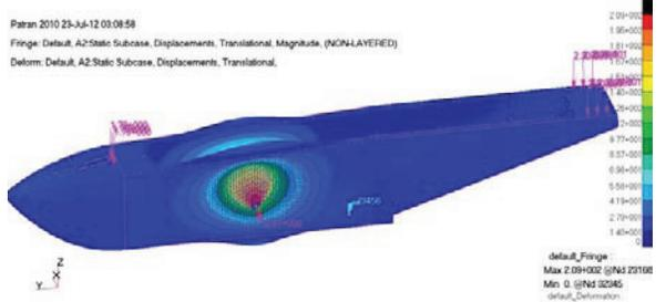
Figure 20. Displacement of Fuselage
