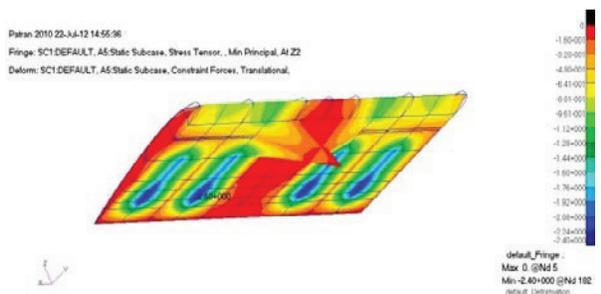
Figure 13. Min. Principal Stress of Horizontal Tail
