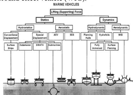
Figure 1. Marine vehicles classification according to supporting force
