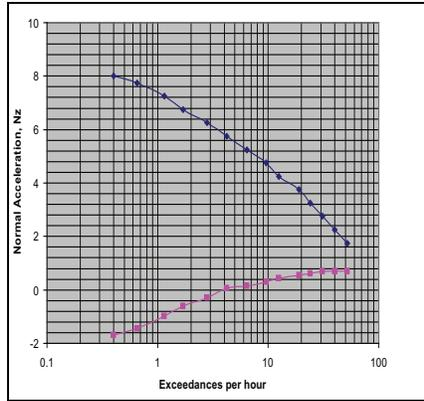
Figure 6. Fatigue Load Spectrum of Typical Trainer Aircraft
