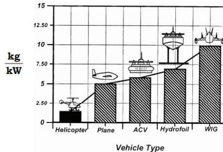
Figure 2. Payload per installed power ratio for different vehicles types.
