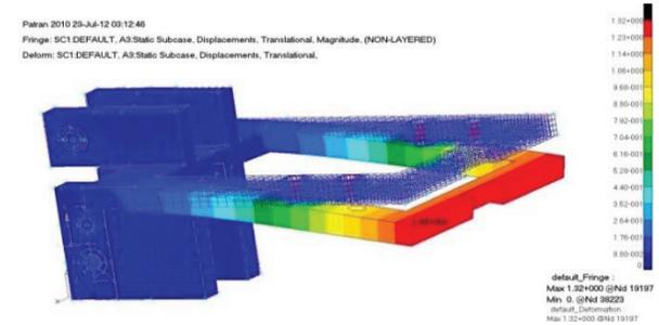
Figure 8. Displacement of Engine Mount
