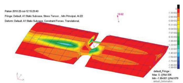
Figure 19. Min. Principal Stress of Wing
