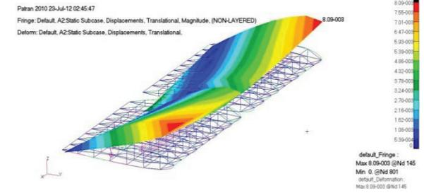
Figure 17. Displacement of Wing
