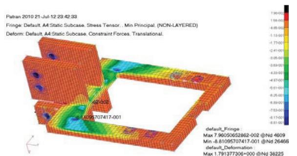
Figure 10. Min. Principal of Engine Mount
