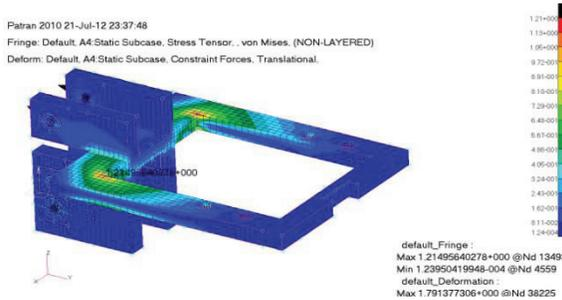
Figure 7. Von mises Stress on Engine mount
