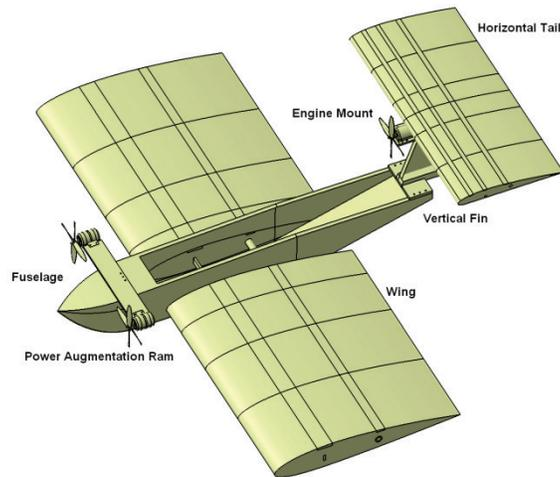
Figure 4. Structure of Wing in Ground Vehicle
